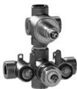
1-745 1/2" Thermostatic Rough-in w/Integrated 2 Way Diverter w/share function ports 1 & 2, & shut off control. Flow rate of 8 gpm at 60 PSI hot and cold mixed flow, top outlet. Factory calibrated comfort setting at 100-deg F, built-in check valves w/service stops. Independent adjustment of temperature & volume control. \$678 — —
