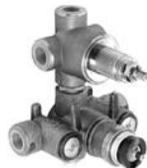
1-744 1/2" Thermostatic Rough-in\*\* w/Integrated 3 Way Diverter & Shut off Control. Flow rate of 6.75 gpm at 60 PSI hot and cold mixed flow, top outlet. Factory calibrated comfort setting at 100-deg F, built-in check valves w/service stops. Independent adjustment of temperature & volume control. \$741 — —
