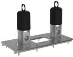
**1-378** Optional Rough For Exposed Tub Filler For subfloor or concrete floor installations. 3.65" overall height. 10.38" x 5" overall base size. Universal 1/2" NPT connections. Test caps included. For use with 3-196 or 3-226 tub risers.
