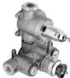
1-742 1/2" Thermostatic Rough-in\*\* w/Integrated 2 Way Diverter & Shut off Control. Flow rate of 10 gpm at 60 PSI hot and cold mixed flow, top outlet. Factory calibrated comfort setting at 100-deg F, built-in check valves w/service stops. Independent adjustment of temperature & volume control. \$678 — —
