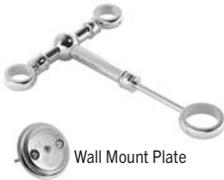
**2-734** Stabilizer Kit for Exposed Tub Floor Riser Kits Adjustable for risers that are 6" to 9" apart. Includes 1-1/2" finished ring for connecting kit to tub overflow pipe. Finished plate for wall mounting up to 10" center of riser pipes.
