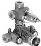
1-743 1/2" Thermostatic Rough-in w/Integrated 3 Way Diverter w/share function ports 1 & 2, & Shut Off Control. Flow rate of 8 gpm at 60 PSI hot & cold mixed flow, combo outlet. Factory calibrated comfort setting at 100-deg F, built-in check valves w/service stops. Independent adjustment of temperature & volume control. \$741 — —
